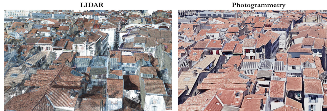
Figure 1. Survey of Petit Bayonne geometry by remote sensing
